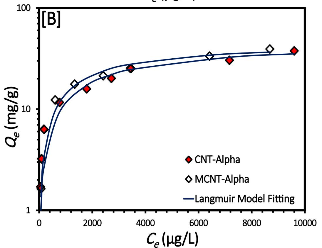
**Fig 8.** The adsorption isotherm of atrazine for [A] CNT-Wako and MCNT-Wako, and [B] CNT-Alpha and MCNT-Alpha.
