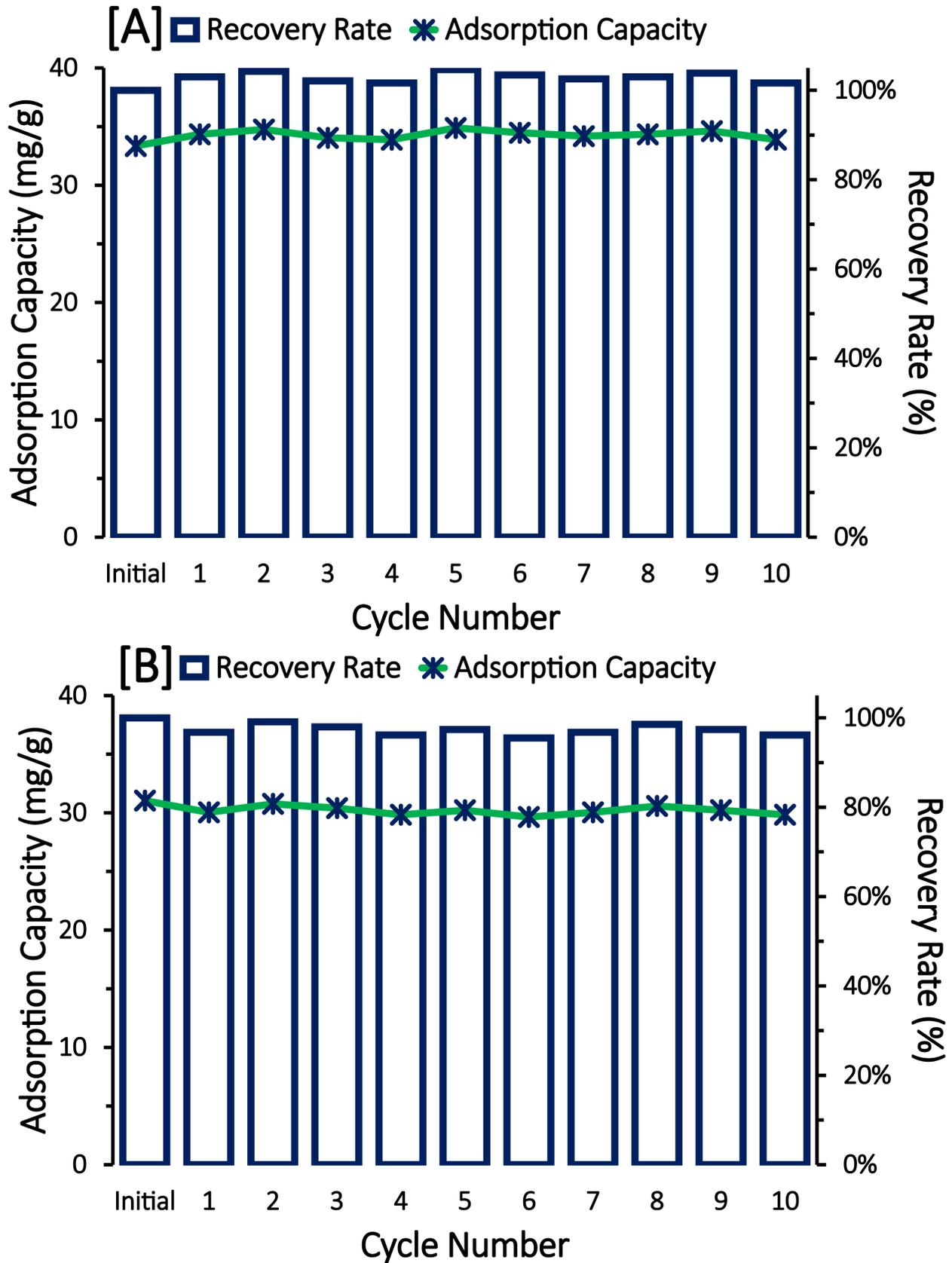
**Fig 9.** Adsorption capacity and recovery rate for [A] MCNT-Wako, and [B] MCNT-Alpha after ten reuse cycles. Initial atrazine concentration was 5 mg/L and MCNT concentration was 500 mg/L at pH  $7 \pm 0.2$  and the equilibrium time at 180 min.
