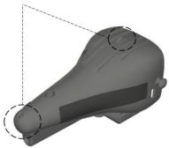
In order to have further influence on the running and sinking behavior, the hollow chamber in the back can remain filled with air, or it can be filled with water or sand; to give an example. Afterwards, the hollow chamber is to be closed with the rubber stopper.
