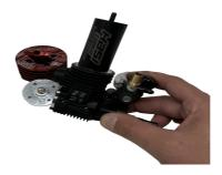
5. Tighten the nut and begin to unscrew. The sleeve will start to come out.
