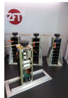
The 4 NetSat Nanosatellites, launched September 2020, to realize formation flight in 3D
