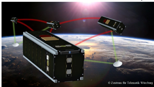
The 4 NetSat Nanosatellites, launched September 2020, to realize formation flight in 3D
