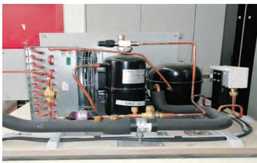
The main cooling system is supplied filled with refrigerant R-513a and is located on top of the device.
