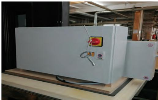
The electricity power should be connected by a specialist. The main control box which has an electrical unit with a red main switch, is located on the device. Use this to switch the device on and off. To get to the main switch, you have to unscrew the inspection flap.
