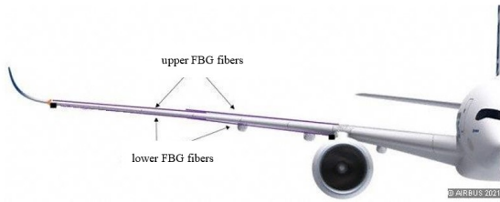
Fig. 11: Schematic diagram of the optical fiber sensors installation on the A350 wing
