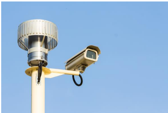
Fig. 1. Security camera with with telemetry module [2]
