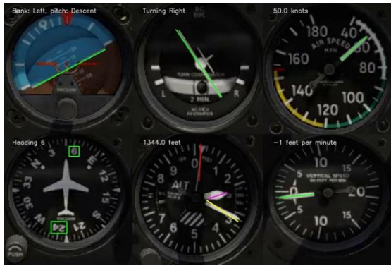
Fig. 6. Cockpit Digitalization (markings in green). Heading: Left/Descent, Turn: Right, Airspeed: 50 Knots, Heading: 6 Degree, Altitude: 1544 Knots, Vertical speed: -1 fpm
