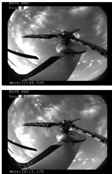
Fig. 2. Camera clearly showing ice accretion on rear rotor blades in 26 seconds thanks to the synchronization of picture capture on the blade frequency.
