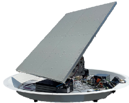
Fig. 1. Picture of Sparte e-100 ground station.
