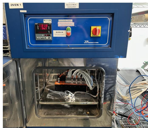
Fig. 10. AXN/CHS/16U/AB2 test article in thermal chamber with thermcouple.
