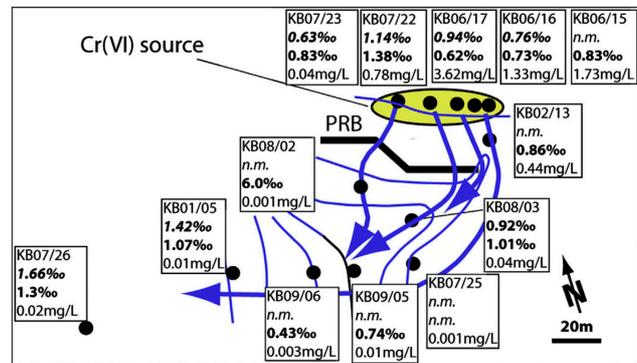
Spatial distribution of measured Cr(VI) concentrations and  $\delta^{53}\text{Cr}$  values of samples collected at the Thun PRB site in September 2010. Also shown is the full interpretation of the hydrologic flow field derived from a multi-tracer experiment, Cr isotope measurements and piezometric elevation contour lines obtained from water table measurements.
