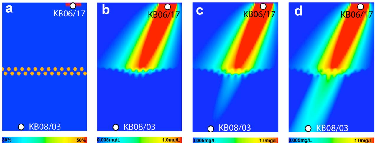
Results of model run performed to simulate the theoretical PRB Cr(VI) breakthrough using the reaction kinetics obtained from column experiments (Wanner et al., 2011): a illustrates the model setup in terms of porosity showing the Cr(VI) source area in red, the PRB domain in yellow and the aquifer domain in blue. Obtained temporal Cr(VI) evolution are shown for 100 days (Fig. b), 150 days (Fig. c) and 200 days (Fig. d).
