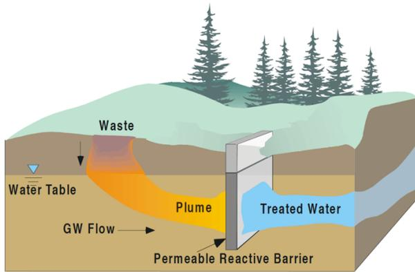
Schematic illustration of the principle of a permeable reactive barrier (PRB). PRBs are filled with an appropriate reactive material and are placed perpendicular to a contaminant plume. From Powell et al. (1998)
