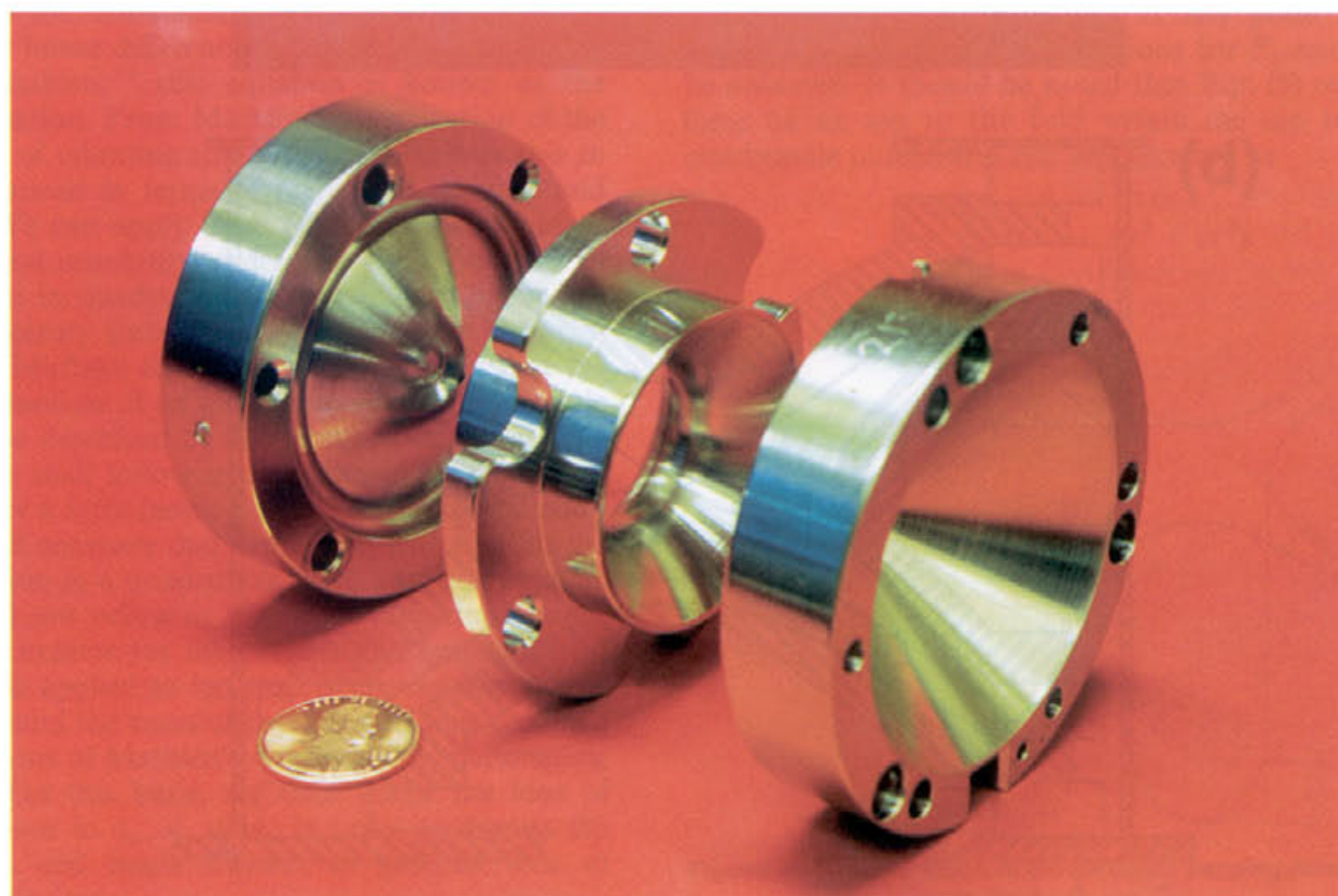
Figure 2. The three electrodes of the quadrupole ion trap shown in open array.
