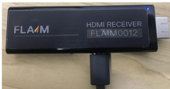
Figure 4 Step 3. Ensure HDMI receiver is powered (Blue light) – top right
