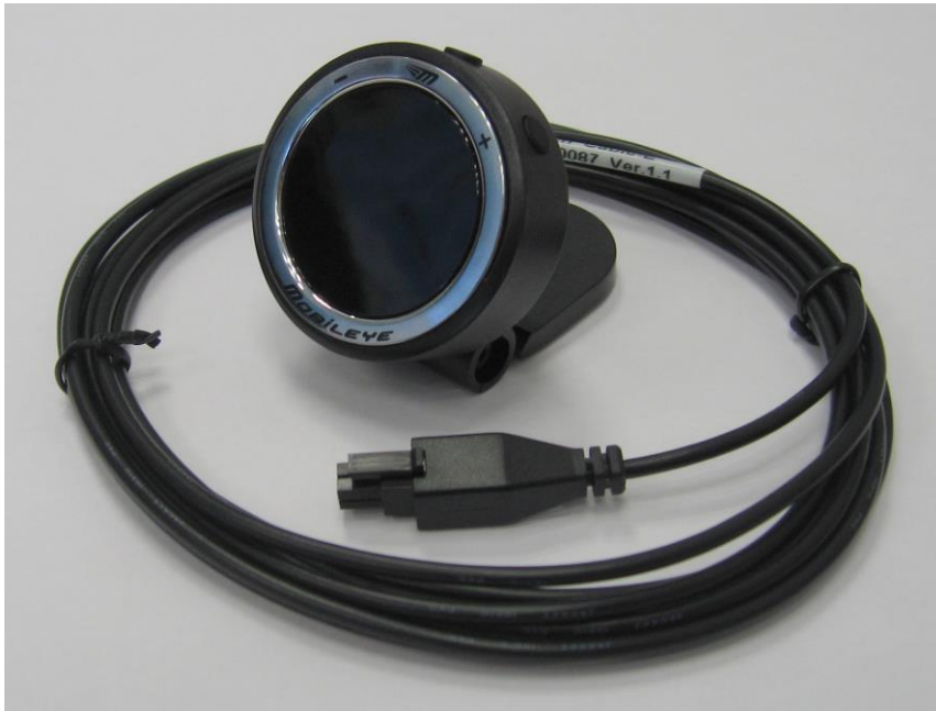
Figure 2: EyeWatch Display and Control Unit with connecting cable
