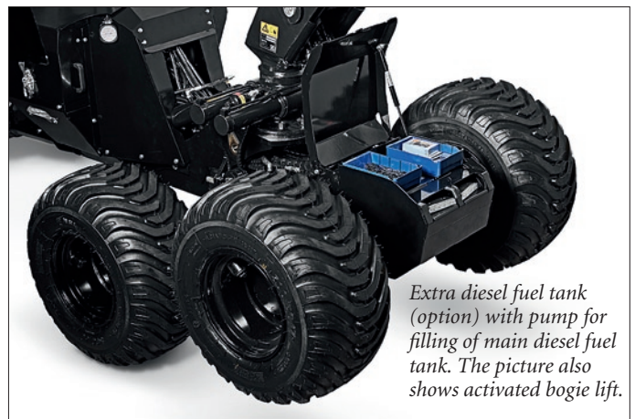
Spacious storage compartment for tools, harvester bars and extra diesel containers (or as shown containers for stump treatment fluids).
