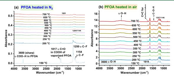
Figure 2. TGA-FTIR spectra of PFOA when heated at various temperatures ranging from 150 to 700  $^{\circ}$ C in N<sub>2</sub> (panel a) and air (panel b) environments.
