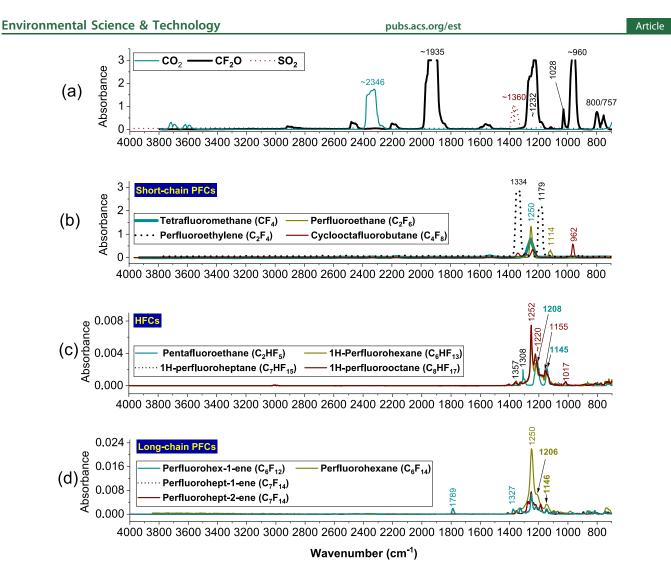
Figure 1. Panels (a–d) display the reference FTIR spectra<sup>118,120–125</sup> for various possible species generated from PFAS during thermal treatments, including short-chain PFCs, HFCs, and long-chain PFCs.
