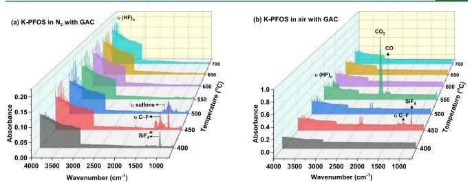
Figure 7. FTIR spectra of K-PFOS subjected to thermal treatment in the presence of GAC in (a)  $N_2$  and (b) air atmospheres at varying temperatures. The peak absorbance values between 4000 and 3000 cm<sup>-1</sup> have been amplified 5-fold to highlight (HF)<sub>n</sub> clusters.
