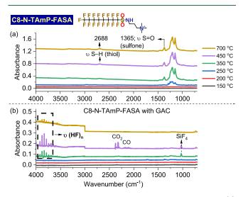
**Figure 6.** FTIR spectra of C8–N-TAMP-FASA heated in air: (a) without GAC and (b) with GAC. To enhance clarity, we have amplified the peak absorbance values between 4000 and 3000 cm<sup>-1</sup> 5-fold in panel (b). The assignments of FTIR peaks for all PFAS analyzed in this study are detailed in Table S2.
