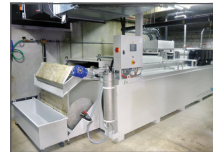
TIEFBETTFILTER / DEEP BED FILTER
