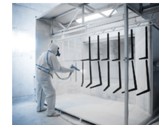
Feinfilter in Farbspritzanlagen Fine filter in paint-spraying units
