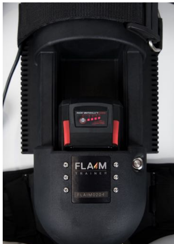
Figure 12 Battery connected and secured
