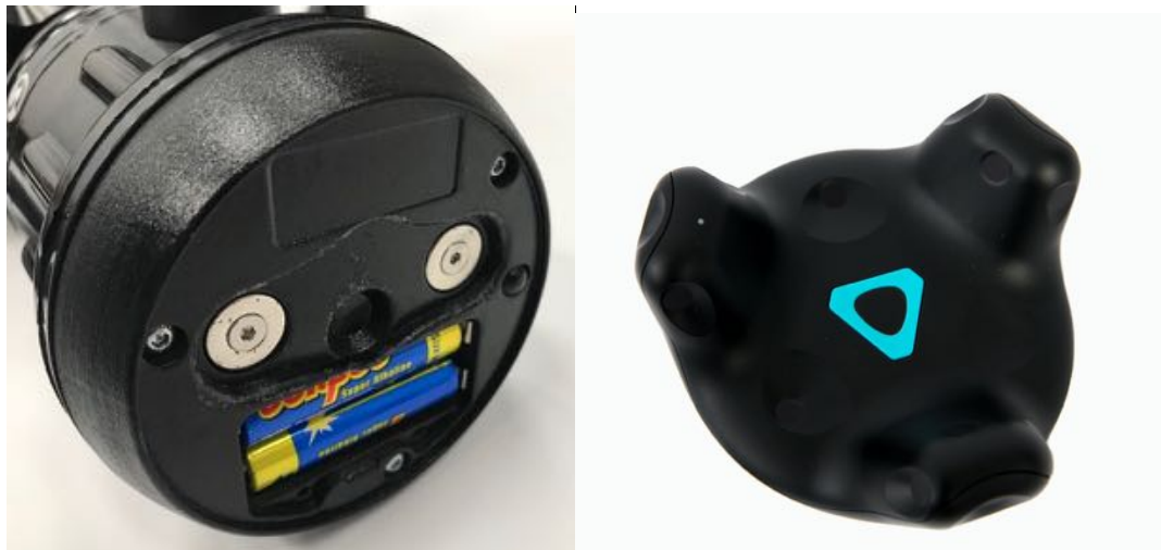
Figure 15 Nozzle face showing batteries installed and tracking puck
