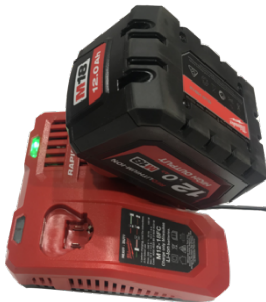
Figure 40 Main battery charger connection
