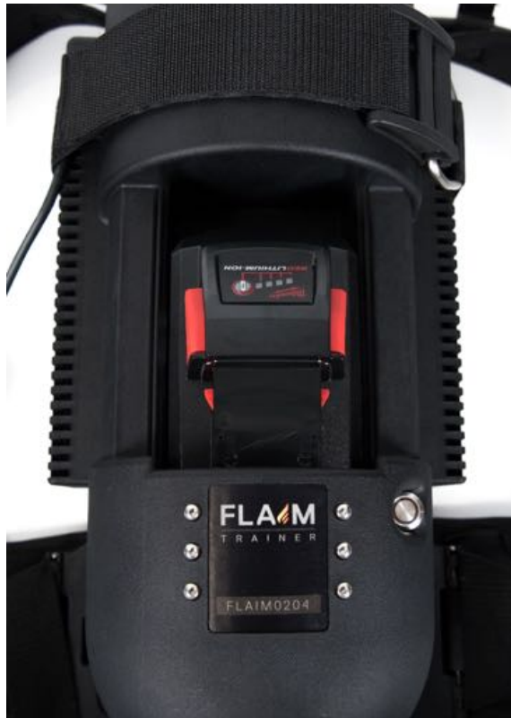
Figure 11 SCBA Main battery installation
