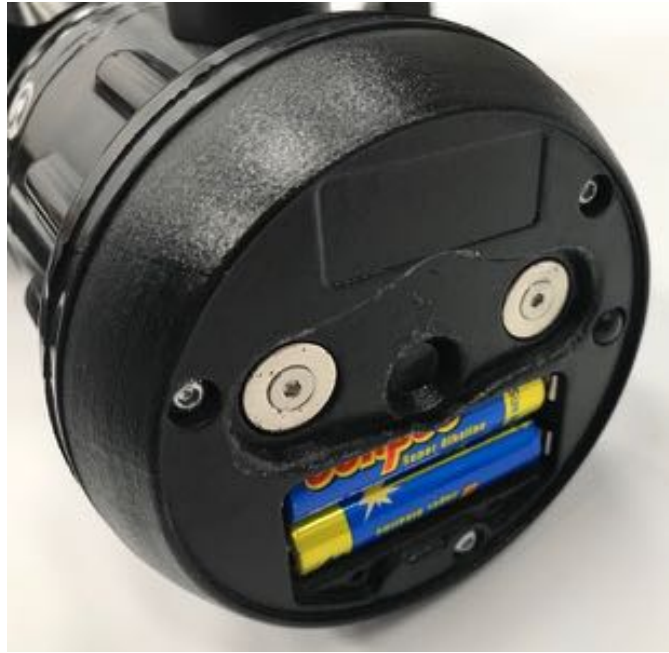
Figure 42 Nozzle batteries behind tracking puck
